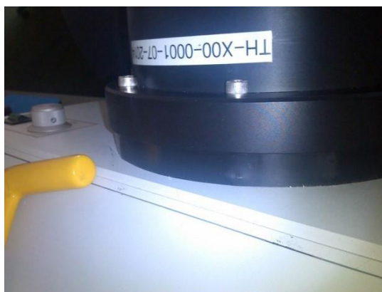
Figure 8: Correctly mounted dome and manifold.
